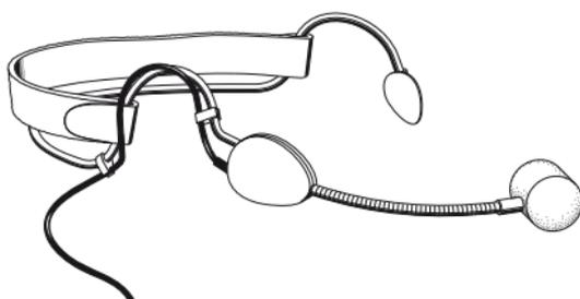
The ME 2 with omni-directional pick-up pattern picks up sound equally from all directions. It is the best choice if movements of the speaker's head have to be compensated for. However, it should be attached as close as possible to the sound source.
