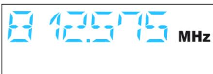
By briefly pressing the **▲/▼** rocker button, the display jumps either forwards or backwards to the next setting. In the "CHAN", "TUNE" and "NAME" menu, the **▲/▼** rocker button features a "fast search" function. If you hold down a button, the display cycles continuously, allowing you to get fast and easily to your desired setting.
