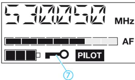
To deactivate the lock mode, first press the SET button and then press the ▲/▼ rocker button to select “LOC.OFF”. If you confirm your selection by pressing the SET button, the buttons can be operated as usual.
