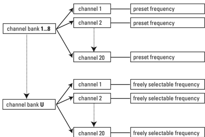
Each of the channels in the channel banks "1" to "8" has been factory-preset to a transmission frequency (see enclosed frequency table). These transmission frequencies cannot be changed but have been preset so that e.g. country-specific regulations on frequency usage are taken into account.
