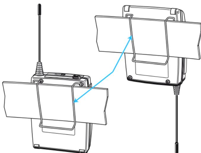
The clip is detachable so that you can also attach the transmitter with the antenna pointing downwards. To do so, withdraw the clip from its fixing points and attach it the other way round.
