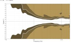
▶ Dispersion angle diagram of a single A15 Focus (left) and A15 Wide (right) in the vertical plane using lines of equal sound pressure at -3 dB, -6 dB, -12 dB.
